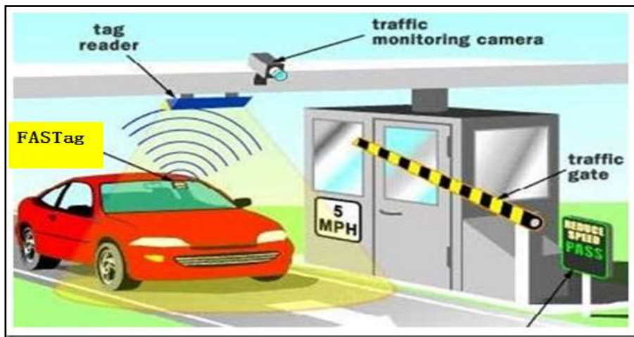
Figure-3: Electronic/Automatic Toll Collection System using Radio Frequency Identification [9]
